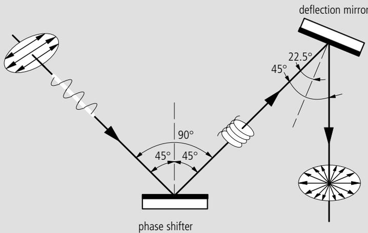
**Phase shifter: the principle is shown above. Below the circular polarizer of a CO<sub>2</sub> laser.**
