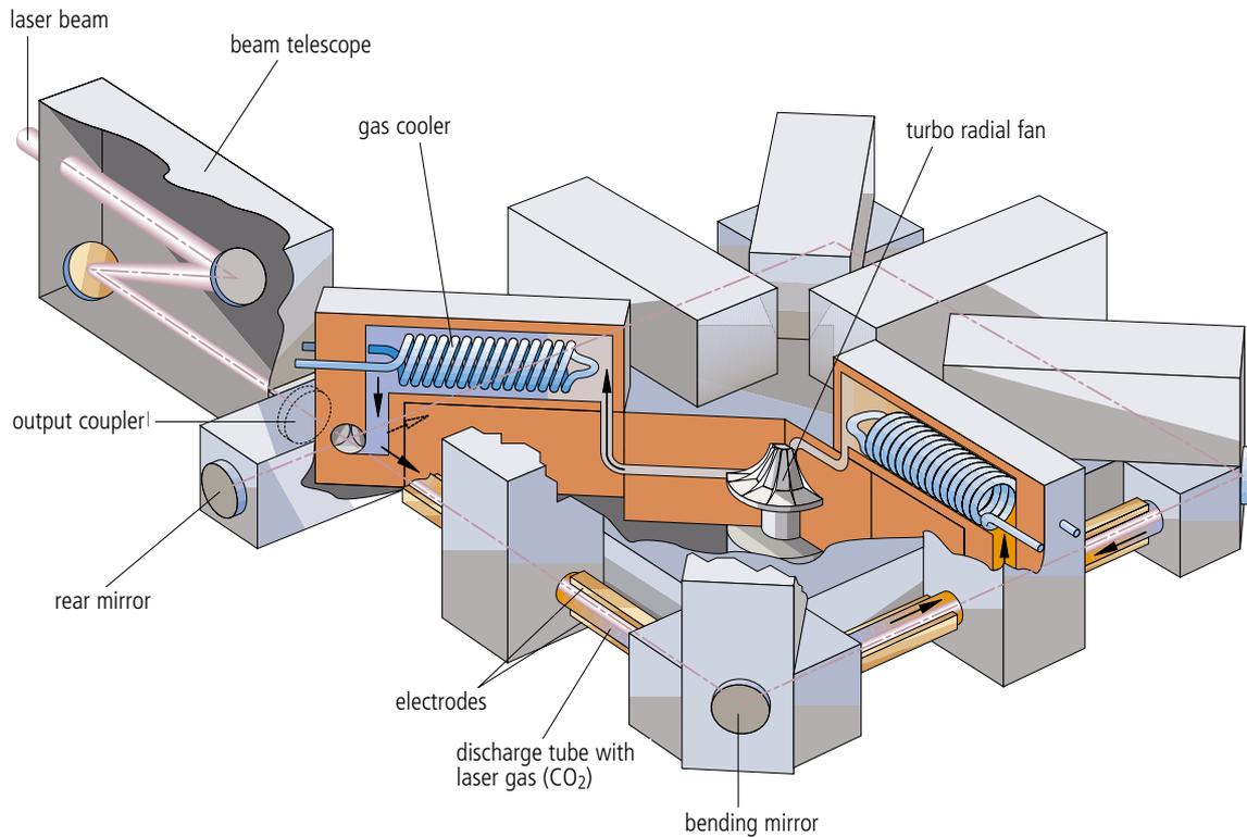
**3. Integrating the laser gas cooling system:** By directly cooling the pump and the gas lines to and from the pump, the laser gas cooling system is made particularly compact.
