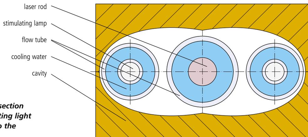
**A double elliptical cross section ensures that the stimulating light is efficiently coupled into the laser rod.**
