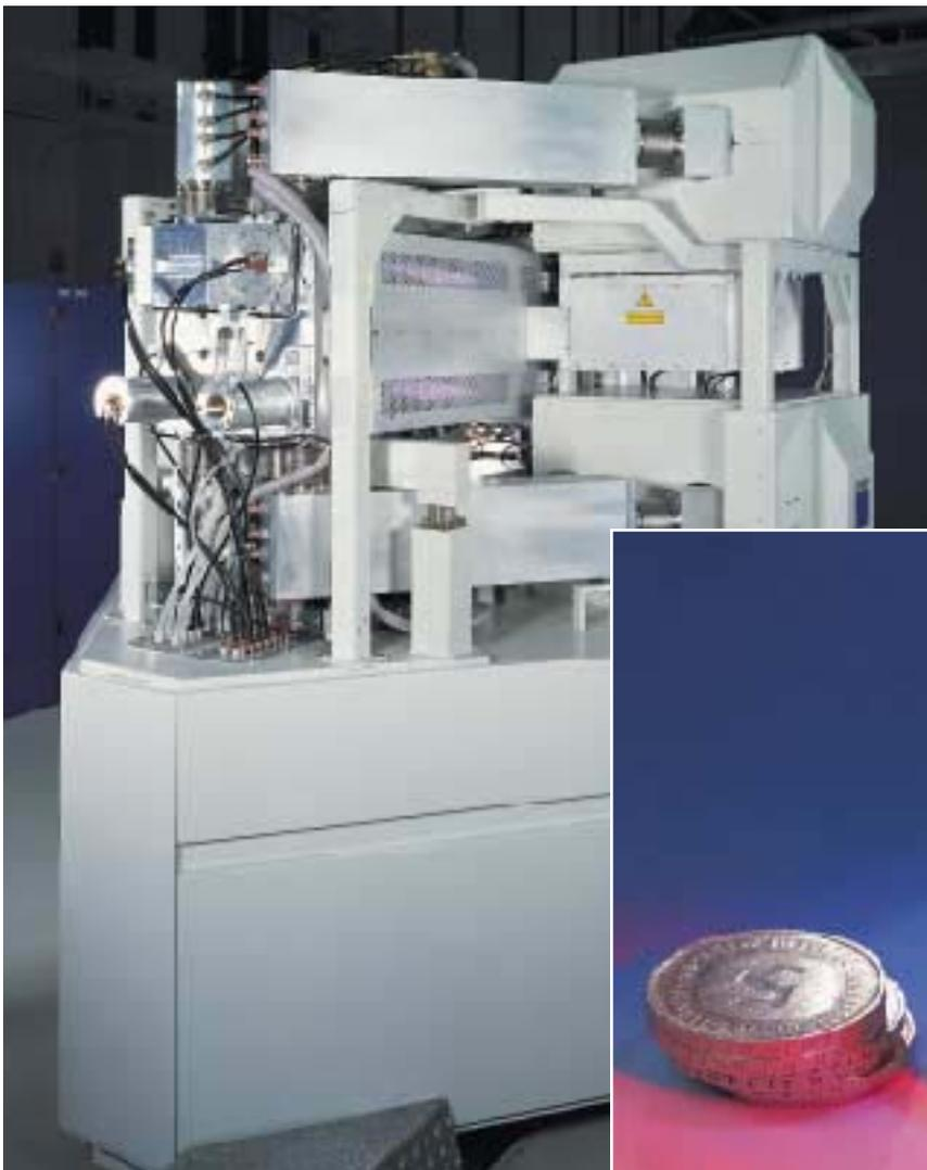
**Large and small high-powered lasers: CO<sub>2</sub> laser (30 kW) and diode laser (200 W)**
