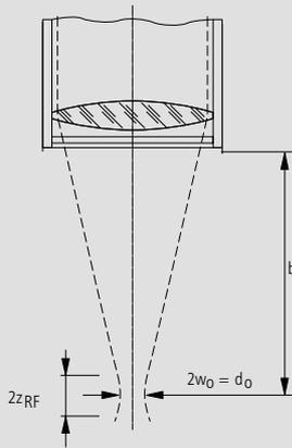
Different variables are used to describe the beam quality. The beam quality of a CO<sub>2</sub> laser is usually indicated by the beam propagation factor K; for an Nd:YAG laser the beam parameter product q. At times M<sup>2</sup> is given. The parameters are defined as follows:
