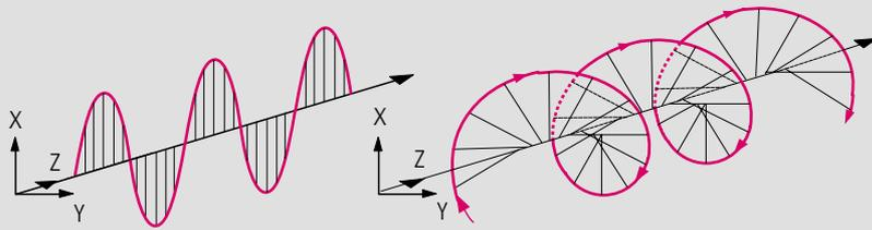
In a linear polarized beam, the electrical field of the electromagnetic waves oscillates only on a single plane (left). In circular polarized light (right) the electric field strength oscillates so that the point of the field vector forms a spiral around the direction of propagation.
