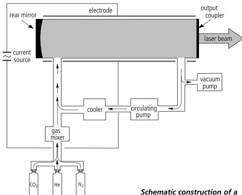
**Schematic construction of a CO<sub>2</sub> laser**
