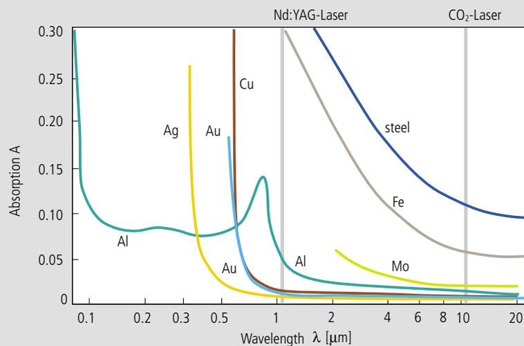
When the laser light strikes the material, only a part of the beam is absorbed. On the one hand, the degree to which the light is absorbed depends on the material itself. On the other hand, it is also dependent on the wavelength of the laser light. The beam of Nd:YAG lasers is absorbed more efficiently than that of CO<sub>2</sub> lasers. This is an important fact to consider when processing precious metals, copper, and aluminum.
