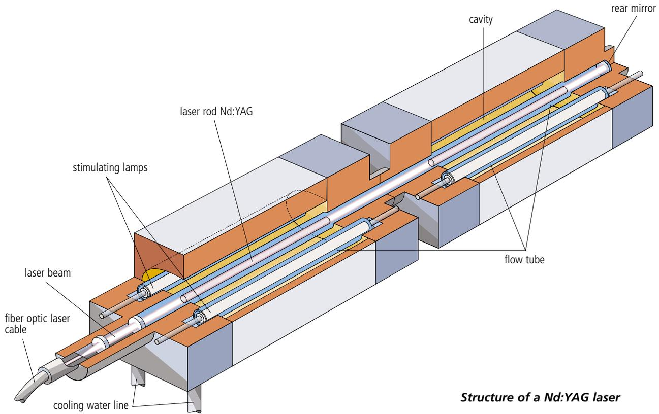
**Structure of a Nd:YAG laser**
