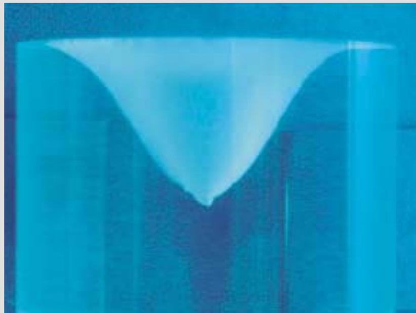
**The intensity distribution in the cross section of a laser beam becomes apparent in the so-called mode shot. The unfocused beam is directed onto the surface of a plexiglas cylinder. This results in the characteristic cavity which has the same shape as the distribution of intensity in the cross section of the laser beam.**
